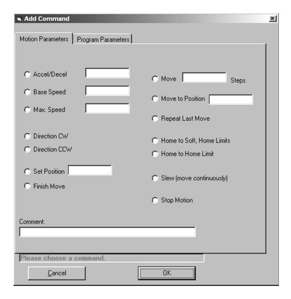
The motion command tab sheet controls the motion information of the motor such as Maximum Speed, Base Speed, Go Absolute, and etc.
